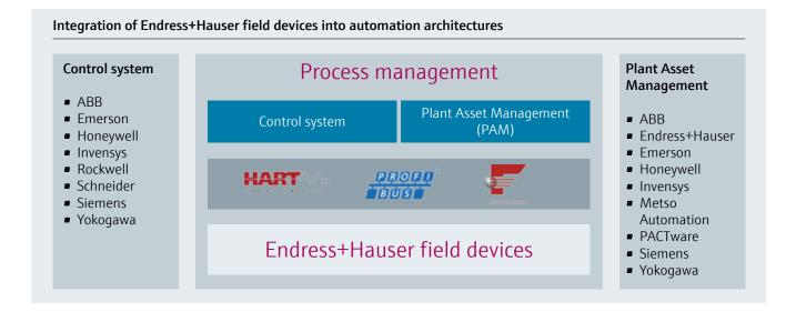
The integration capability of the instruments is tested at our system laboratory thus ensuring their system independence. We also offer training opportunities directed especially to the integration of instruments into respective control systems.
